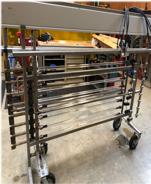
UV Rack Rebuild
