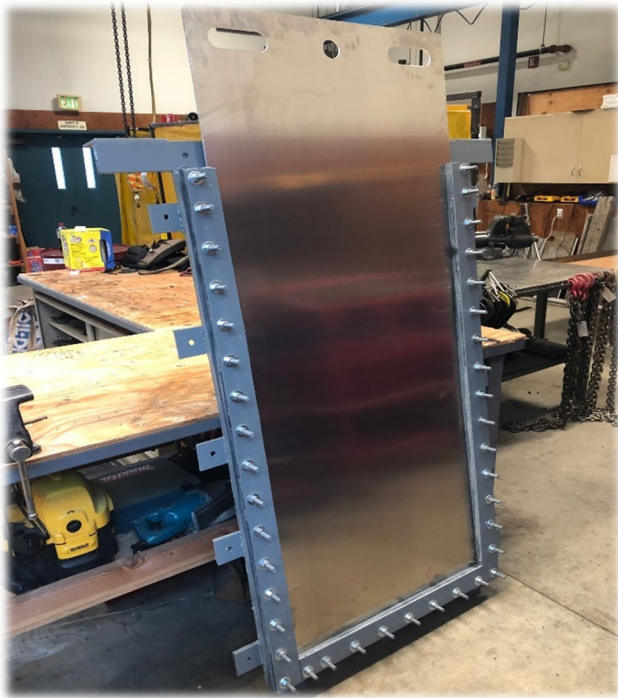
UV stop gate fabrication complete
