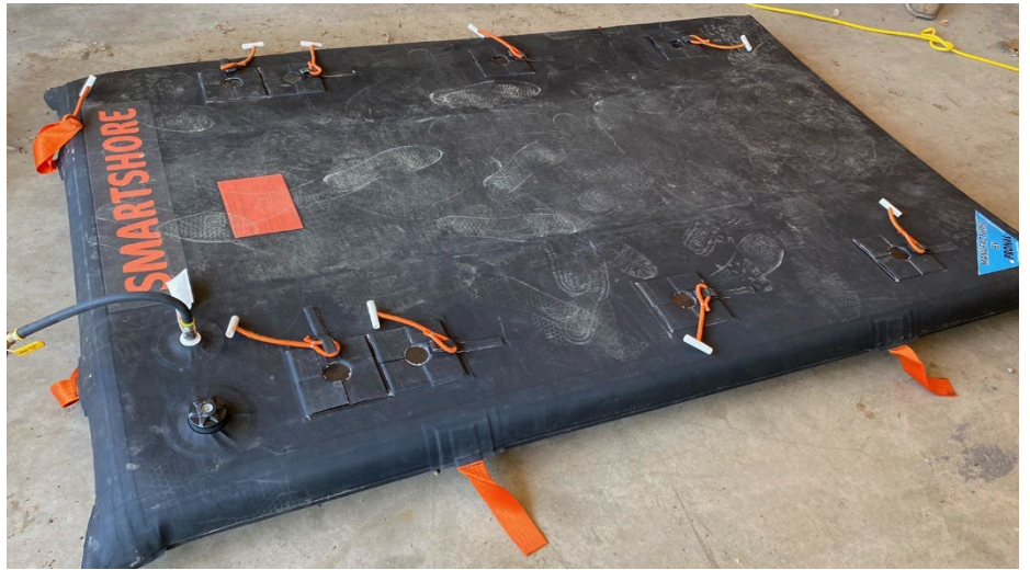
Photo 8: New type of inflatable trench shoring panel
