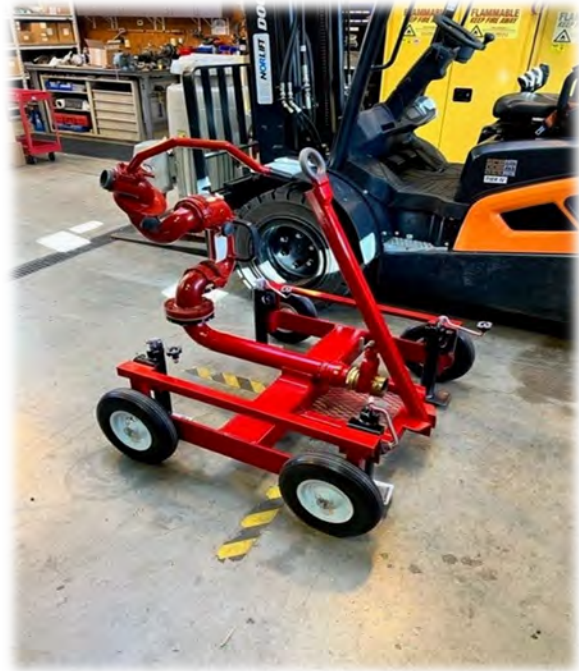
New Fire Monitor for Wetwell Cleaning.
