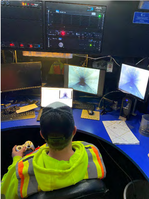
Inside TV Van for Inspection
