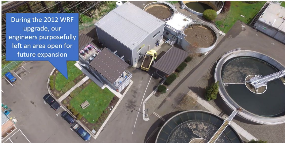
Figure 6-6: Site Footprint Allocated for Future Tertiary Filters
